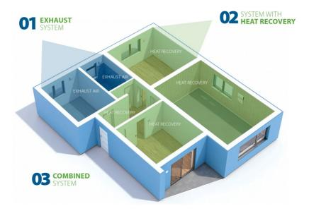
With hybrid ventilation, all living rooms in the residential unit are equipped with e<sup>2</sup> type heat recovery units. The exhaust air rooms, such as the kitchen, bathroom or WC, are vented with an exhaust air unit.
